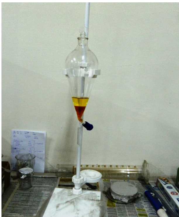
Figure 4.2. Biodiesel(top) and glycerol(bottom layer) Figure 4.3. Biodiesel after removal of glycerol
