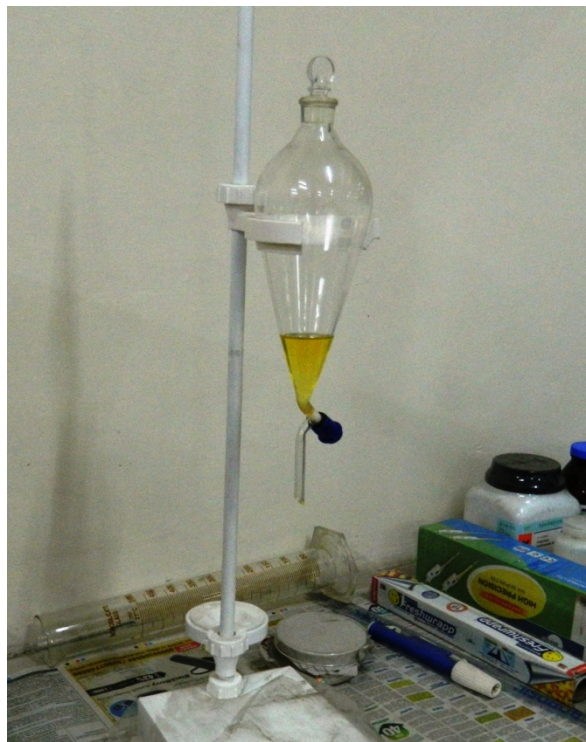
Figure 4.2. Biodiesel(top) and glycerol(bottom layer) Figure 4.3. Biodiesel after removal of glycerol
