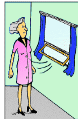
Figure 8: unwanted cooling, due to draught ( http://www.scientificassociates.8m.com/ )
