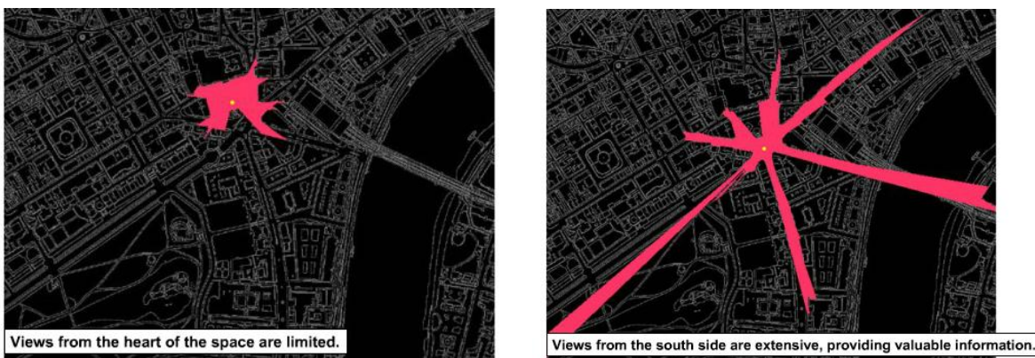
Figure 3.6 Axial Map of Trafalgar Square in London Depicting Isovists Formation at the heart of the space as well as the south side
