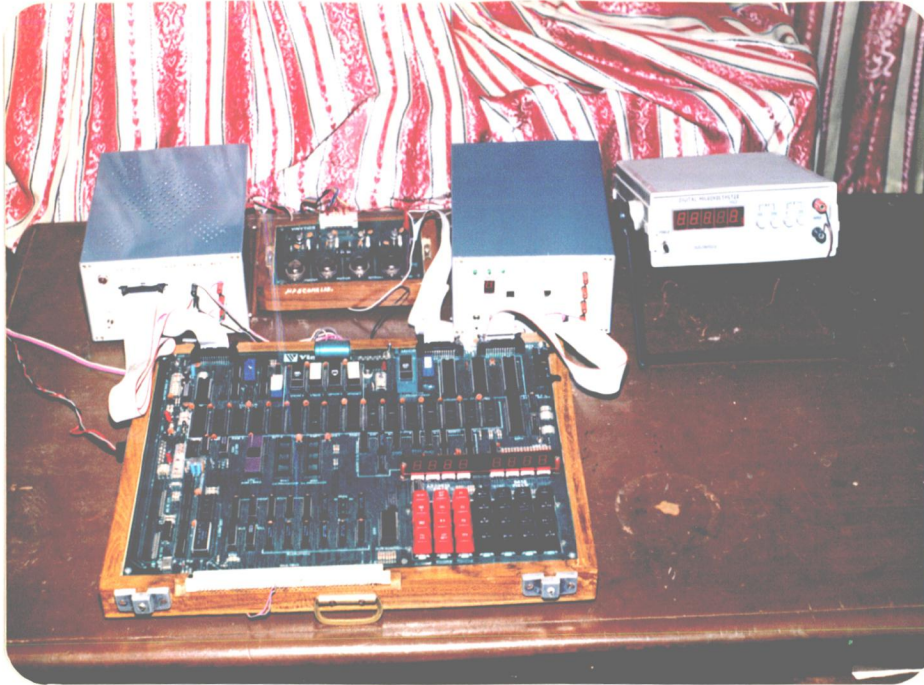
6-7. 8086 \mu p KIT WITH SCR FIRING CIRCUIT MODULE, ADC MODULE AND STEPPER MOTOR DRIVER CARD
