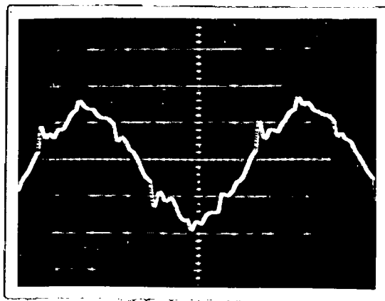
11 . LCI OUTPUT VOLTAGE WAVEFORM WITH CAPACITORS CONNECTED IN PARALLEL .
