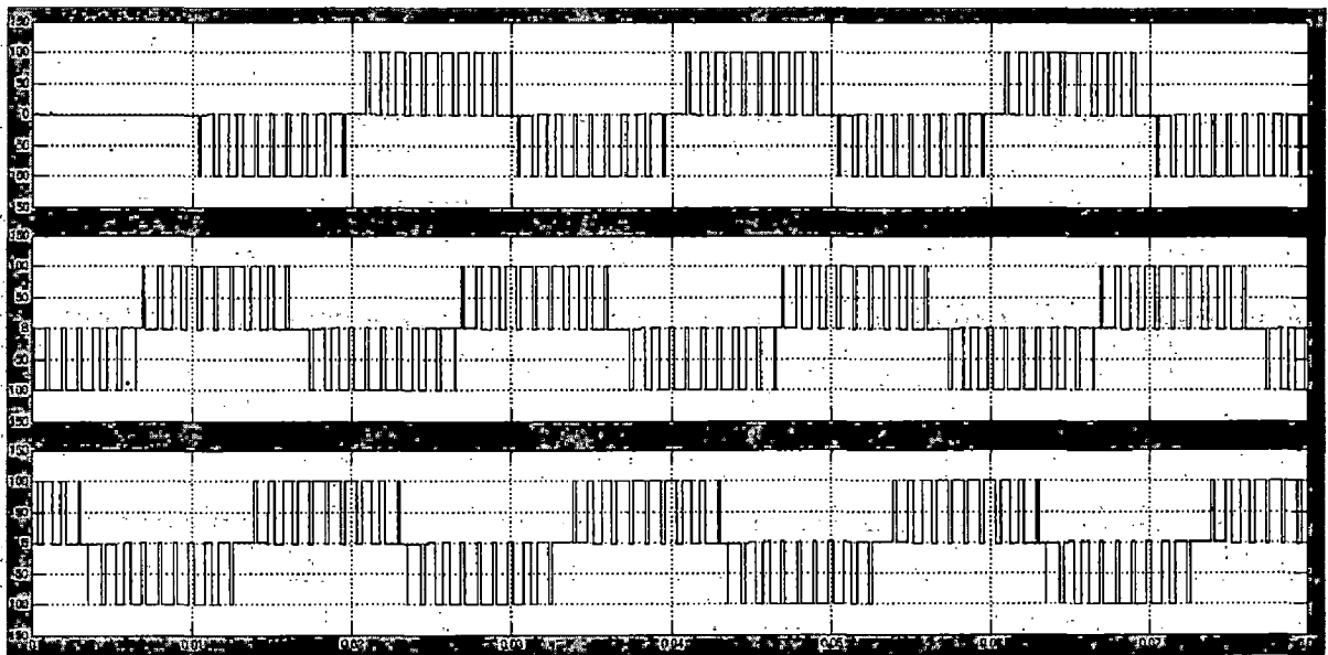
Fig.5.11 Phase-to-neutral voltage wave form without fault diagnosis system i) V_{An} ii) V_{Bn} iii) V_{Cn}
