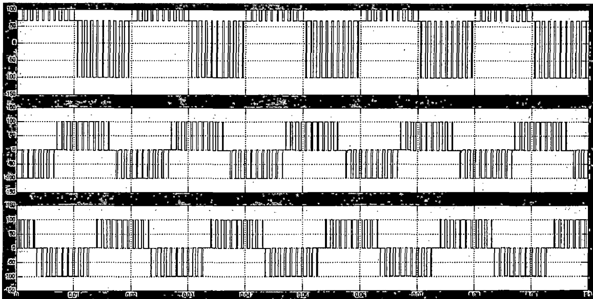
Fig.5.16 Phase-to- neutral voltage waveforms of after the occurrence of fault i) V_{An} ii) V_{Bn} iii) V_{Cn}
