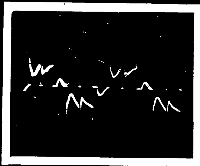
Out-put current of 3- \phi Inverter at 50 c/s with induction motor load.
