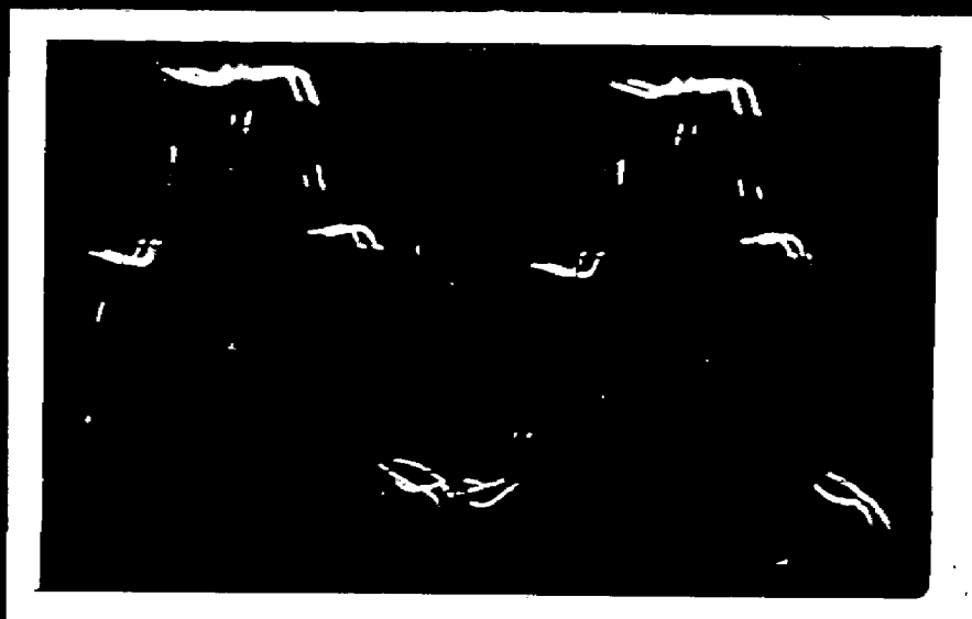
Out-put voltage of 3- \phi Inverter at 16 c/s with induction motor load (a. phase).
