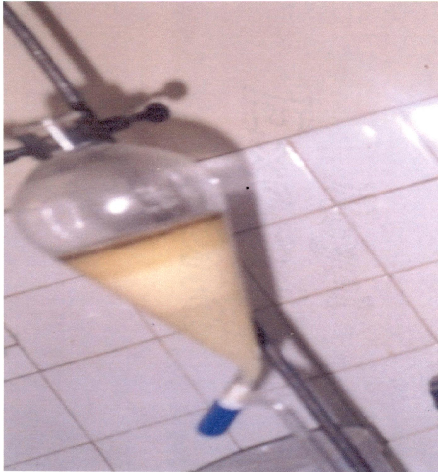
Fig.3.4: Unseparated Emulsion of Biodiesel and Water
