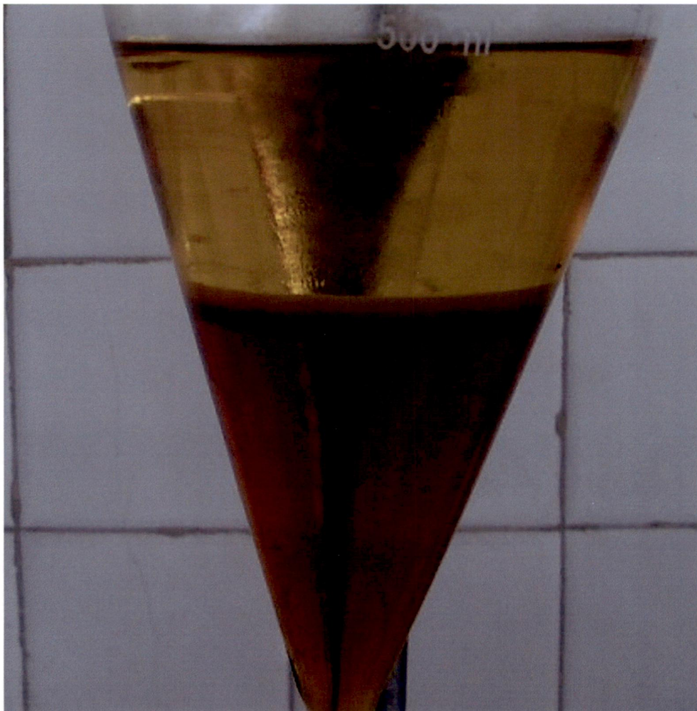
Fig. 3.3: Separated Layers of Biodiesel and Glycerin
