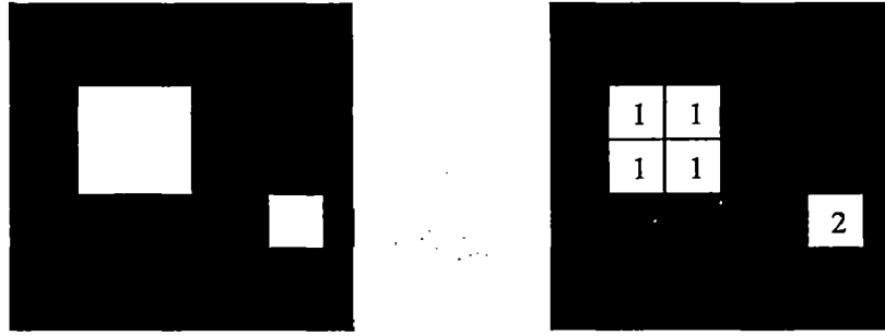
Figure 6.5: Output after applying CCL to an image
