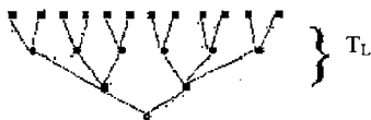
Fig.3.3 Lower tree T_L of a turbo-like LDPC code with column weight 3, row weight 4, and height 4 [19]
