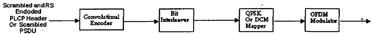
Fig 4.5 Encoding process for the scrambled, Reed-Solomon encoded PLCP header or Scrambled PSDU
