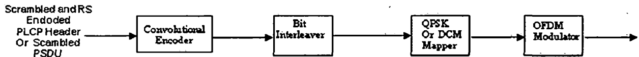
Fig 5.2 Encoding process of scrambled and RS Encoded PLCP Header or Scrambled PSDU
