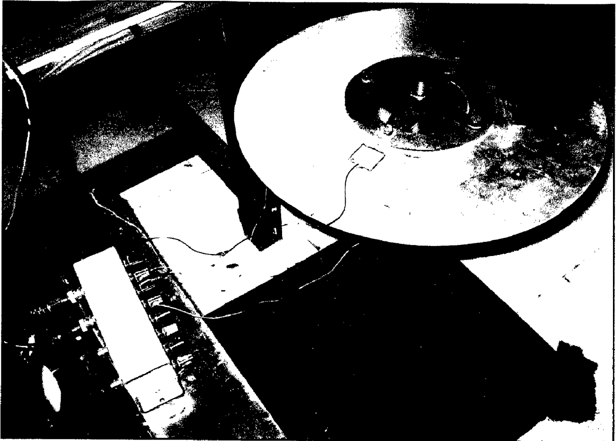
Figure 5.3: Aluminum plate clamped at the inner boundary with PZT patches.
