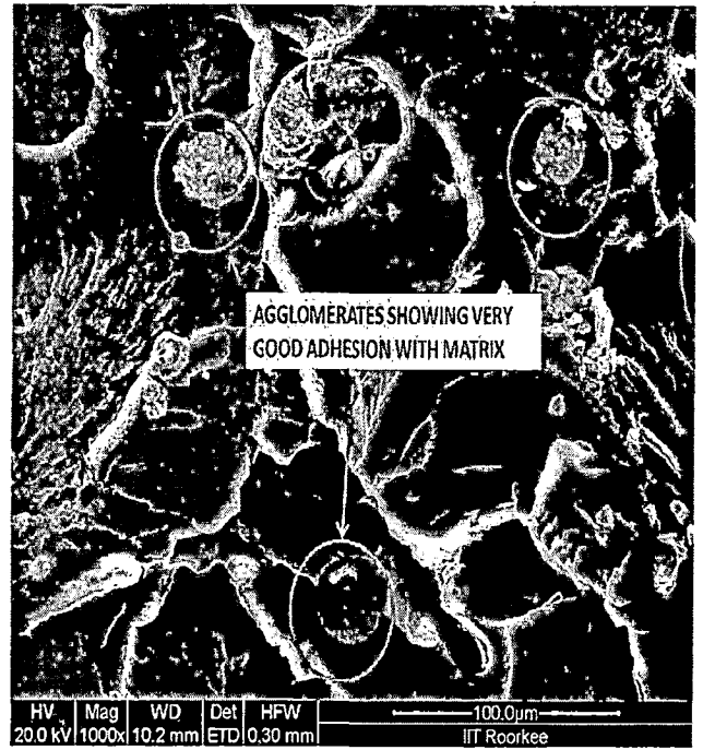
Figure 69:- Fracture surface image of 10 wt.% mech. Mixed composite
