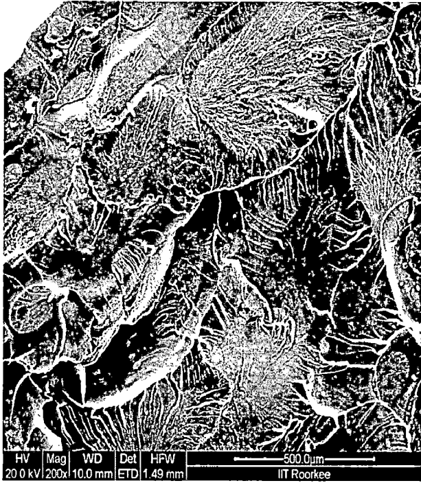
Figure 64:- Fracture surface image of pure epoxy
