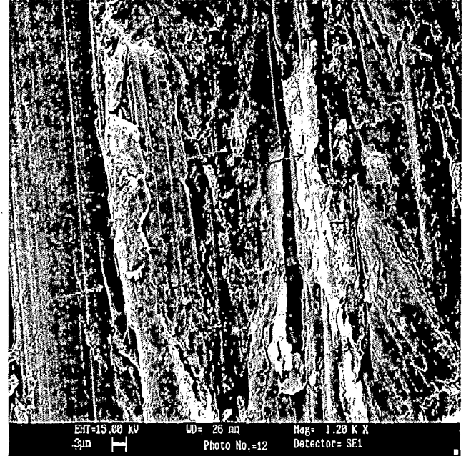
Fig. 89:- Fracture image of 8 wt.% ultrasonically mixed composite (Lap Shear specimen)
