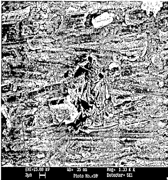
Fig. 88:- Fracture image of 6 wt.% ultrasonically mixed composite (Lap Shear Specimen)
