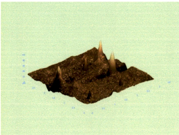
Fig 25. 3D AFM image of 4 wt.% Mech. Mixed composite
