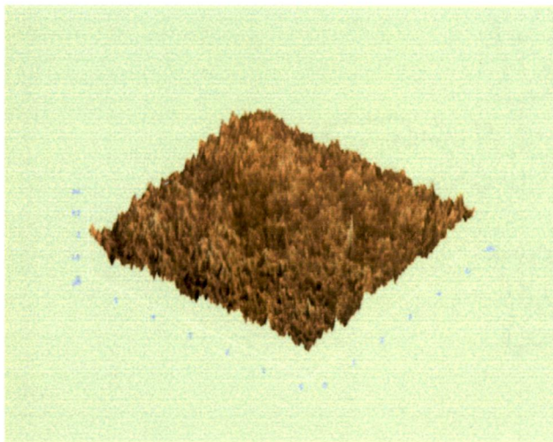
Fig 19. 3D image of pure epoxy
