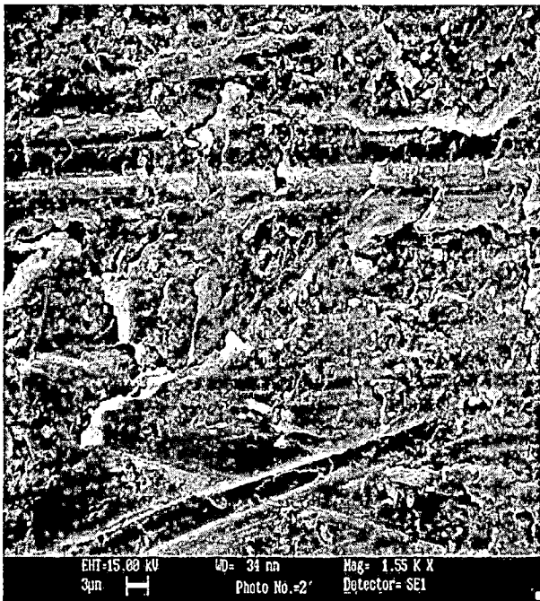
Fig. 84:- Fracture surface image of 20 wt.% ultrasonically mixed composite at higher magnification
