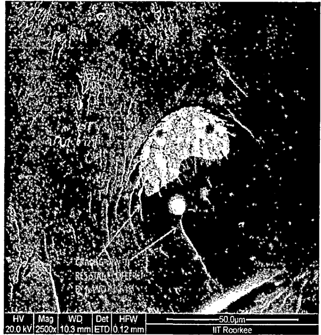
Figure 73:- Fracture image of 20 wt.% mech. Mixed composite at higher magnification
