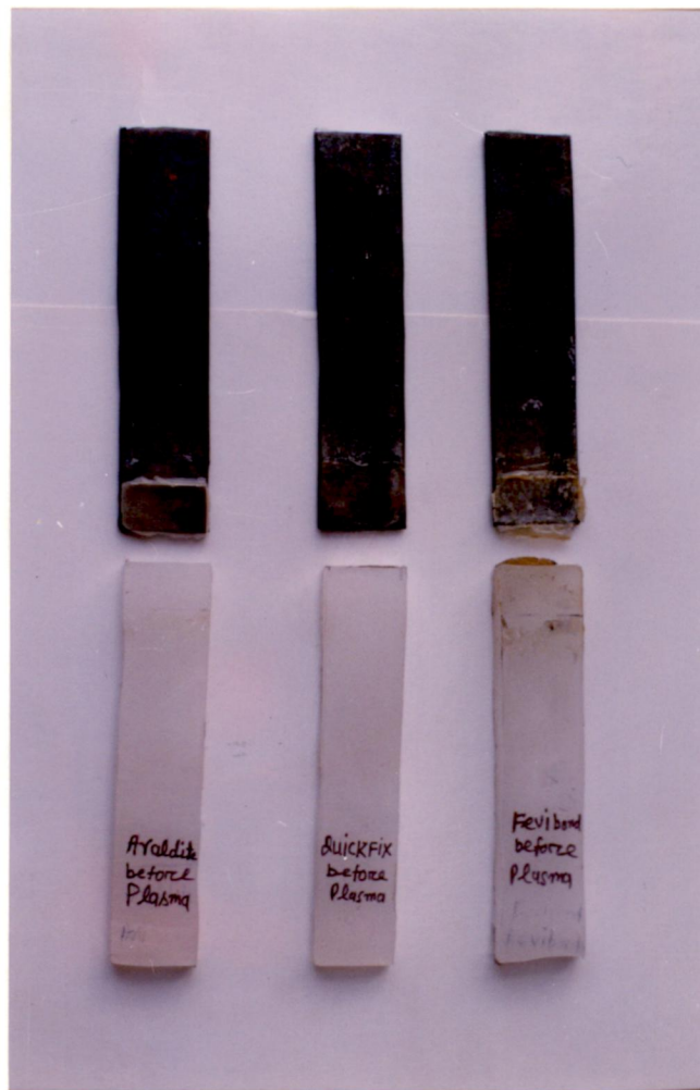
Fig. 4.12 : Failure of adhesive joint of PP to mild steel before glow discharge
