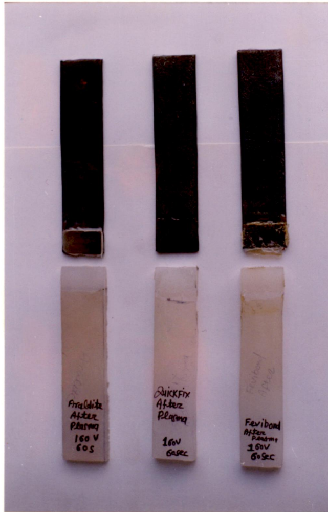
Fig. 4.13 : Failure of adhesive joint of PP to mild steel after glow discharge
