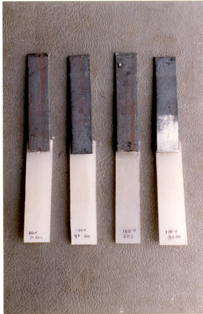
Fig. 4.11 : Adhesive joint of PP to mild steel of different exposure time of glow discharge
