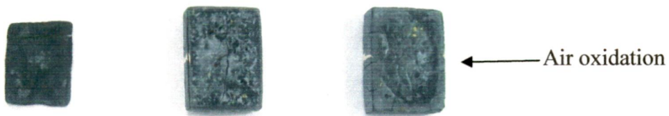
Fig.4.13: Samples after hot corrosion test from left un-weld sample, base metal and weld metal.
