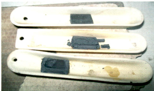
Ceramic boats containing samples.
