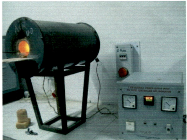
Fig.4.12: Tubular furnace used for corrosion test.
