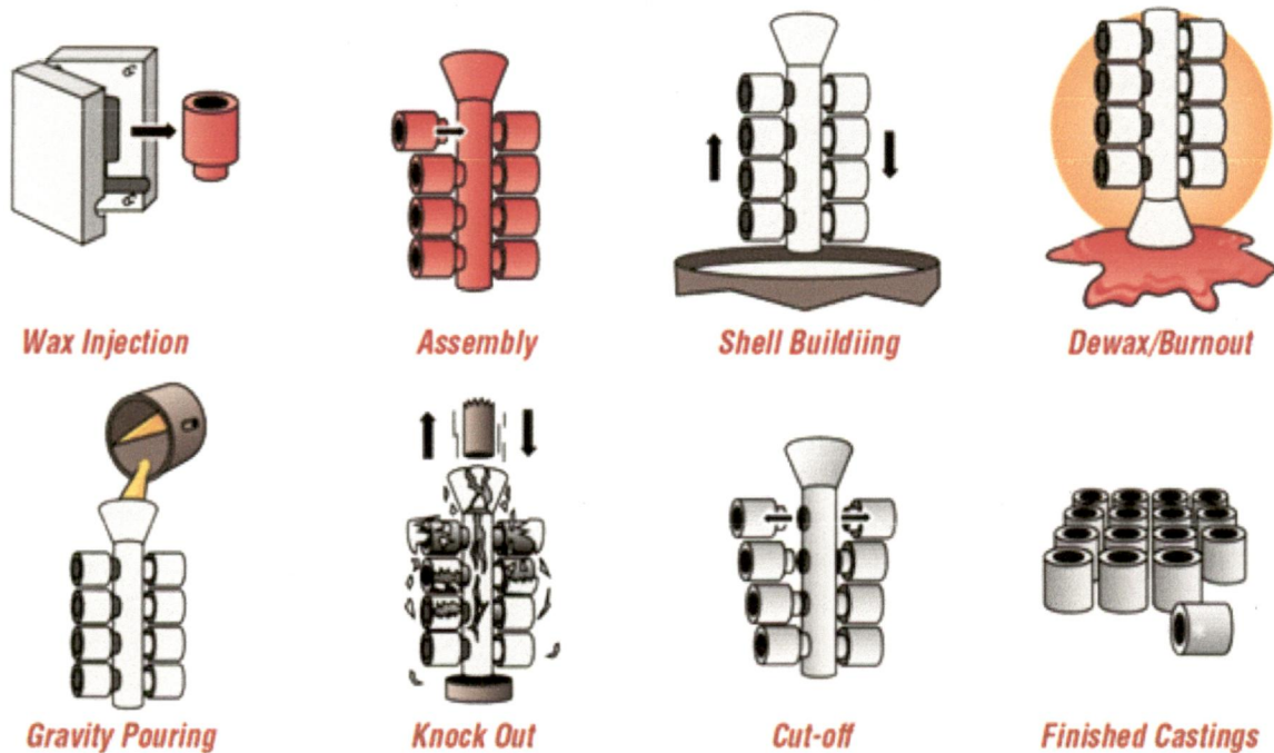
Fig. 1.2: The basic steps in the investment casting process
