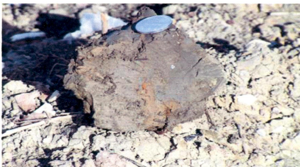
Figure 18: Marine derived tsunami sediment. Note the iron oxide stains and massive structure.
