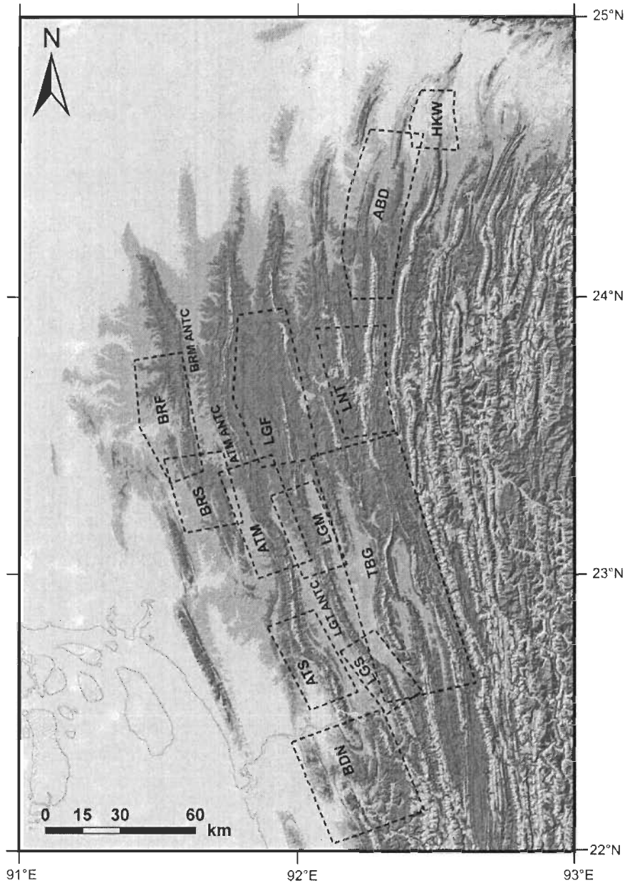
Figure 2. Colour-coded 90-m SRTM-DEM of the study area showing N-S trending linear fold ridges with westward curvature. Grey to red colours represent lowest to highest elevations. Hill-shade prepared from the DEM using sun azimuth 315^\circ , sun elevation 45^\circ and z factor as 0.00000956 and overlaid on the DEM. Colour codes assigned to different height ranges. ATM-ANTC—Atharamura anticline, BRM-ANTC—Baramura anticline, LGT-ANTC—Langtarat anticline, HKW—Hailakandi-west overlap, ABD—Abdullapur overlap, BRF—Baramura west limb fault, LGF—Langtarat west limb fault, BRS—Baramura south overlap, ATM—Atharamura middle, ATS—Atharamura south, LGM—Langtarat middle, LGS—Langtarat south, TBG—Tuibangadam synclines, BDN—Bandarban nose.
