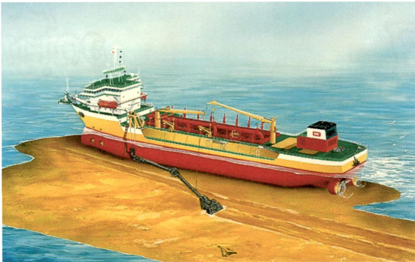
FIG. 1: A SKETCH SHOWING DREDGING OPERATION
