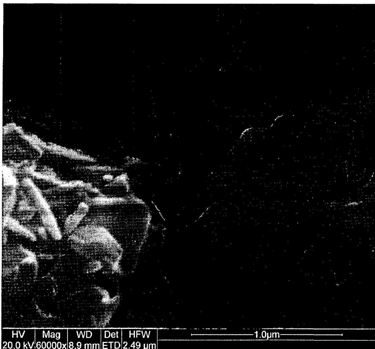
Figure 5.9 FESEM micrograph of ZnO synthesized by using Citric Acid Monohydrate as capping agent.
