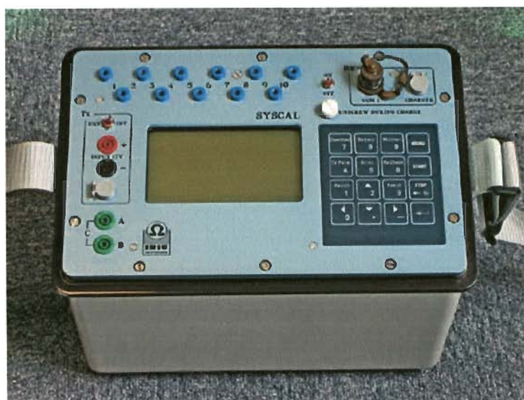
Plate 3.1 Electrical Resistivity Imaging System (IRIS)
