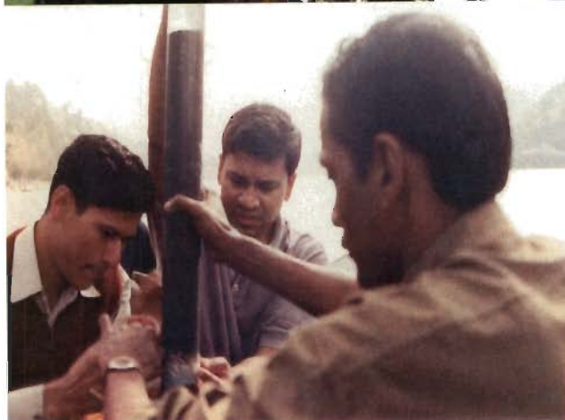
Retrieval of sediment core
