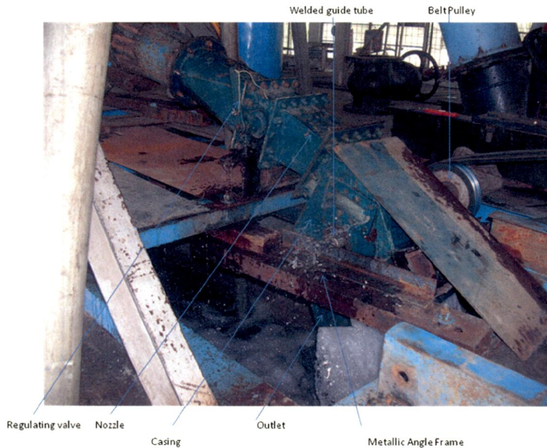
Fig: 5.4 View of full assembly of cross flow turbine at test rig
