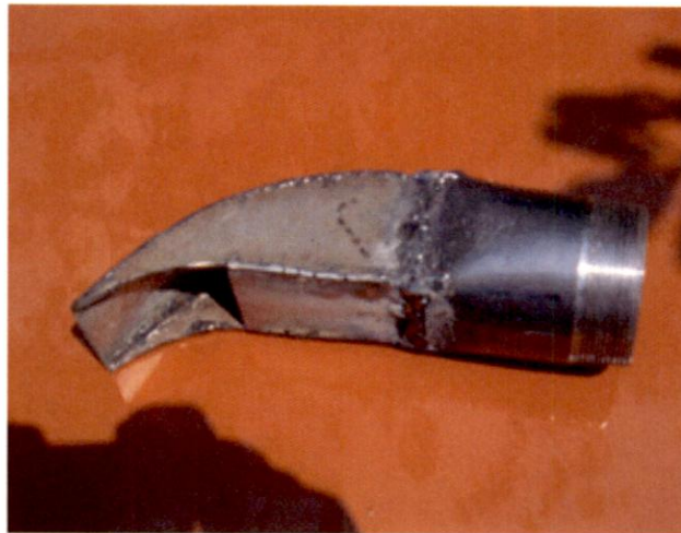
Fig. 3.4: Nozzle of Cross flow turbine [24]
