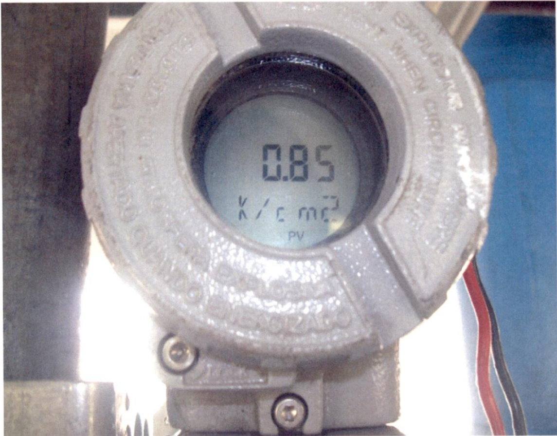
Fig. 5.5: Intelligent Pressure Transmitter, LD301 used for Measuring Head in atmosphere
