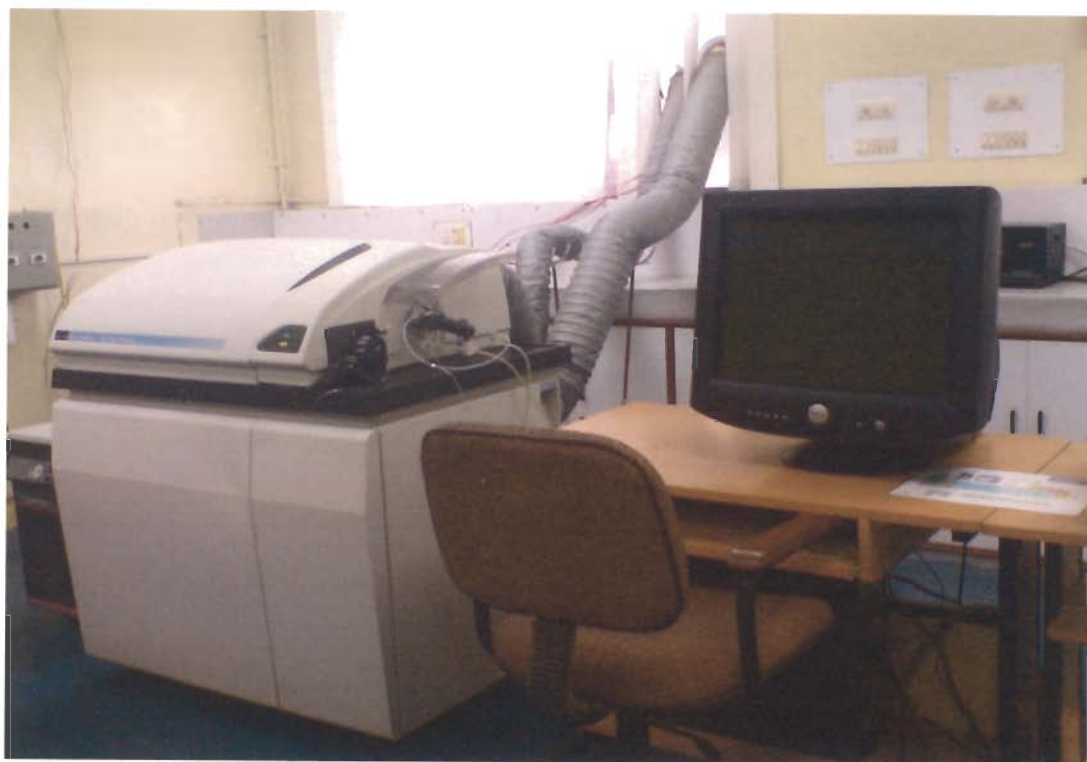
Figure 3.4 ICP-MS (Perkin Elmer, Elan DRC-e) at Wadia Institute of Himalayan Geology, Dehra Dun.
