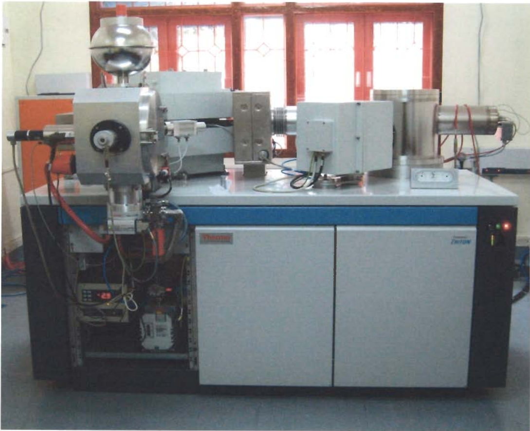
Figure 3.5 Thermal Ionization Mass spectrometry (TIMS, model: Triton-Thermo Finnigan) at National Facility for Geochronology and Geosciences, Pondicherry University, Pondicherry.
