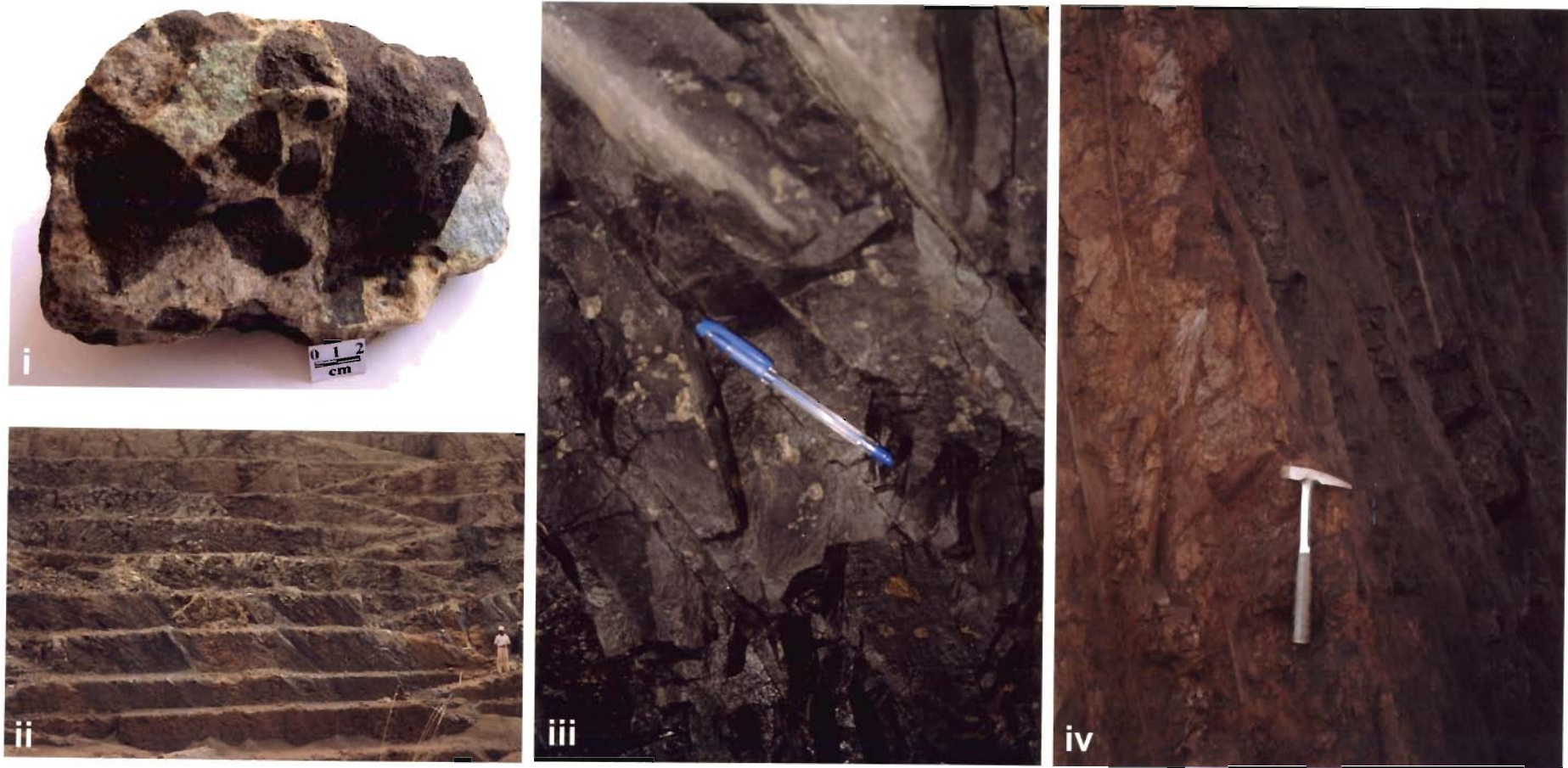
Fig.2.3.i Brecciated chromite, ii minor folds in chromite band, iii serpentinized host ultramafics, iv limonitized host ultramafics
