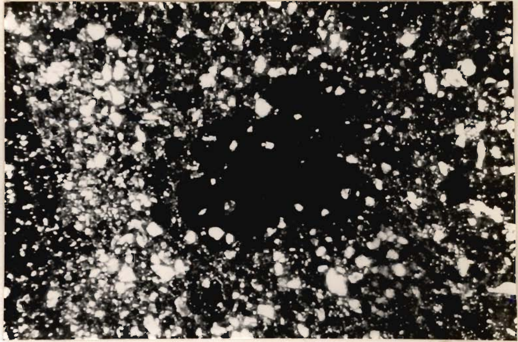
Fig. 4.9 Quartz grains are surrounded by fine material which bridges the voids i.e. Pellicular grain microstructure, Horizon B2, Pedon #P3, Older Piedmont Plain (XPL).
