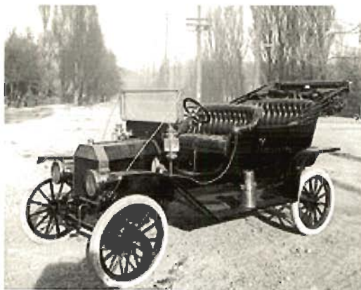
Figure 1.2. 1910 “Ford Model T” where chassis of the car has vanadium containing steel. Source Wikipedia.
